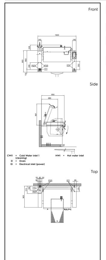
Electric Supply voltage: 400 V/3N ph/50/60 Hz **Total Watts:** 20.6 kW Water: Drain "D": 1/2" Installation: FS on concrete base;FS on
